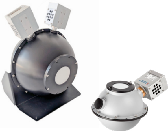
▲ Figure 1: Left: Light source with a 75 mm emitting aperture and a sun-like spectrum. Right: Light source with a 50 mm emitting aperture for more compact setups.
