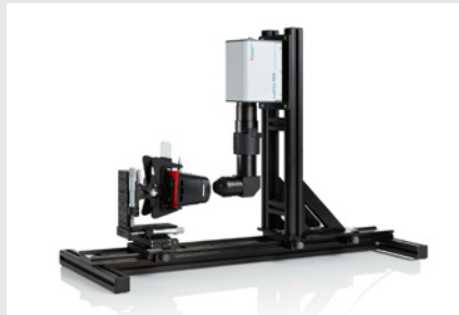
LumiTop AR/VR imaging light measurement device
